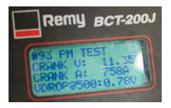
Detail results of the cranking system including:
