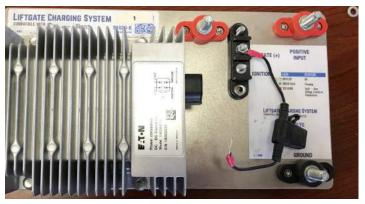
Step 3: Install the new harness by inserting the connector and securely attaching each ring terminal to the plate with the nuts removed in Step 1.
