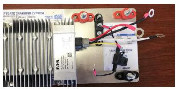
Step 2: Press the clip on the side of the connector and remove.
