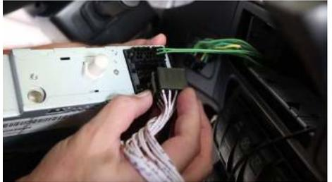
Step 5: Plug the truck wiring harness into the back of the Aware.
