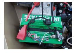
Step 9: Drill two 3/16" holes in the battery handle and use zip ties to secure the LED indicator in place.
