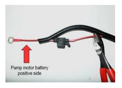
Note: If the circuit breaker holder is still connected to the pump motor battery, pull the circuit breaker to avoid cutting a live wire.
