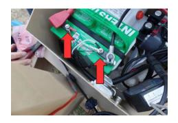
Step 8: Install the BOSS LED indicator by connecting the positive side of the LED (this is the side that the 15 amp fuse is on) to the positive post of the pump motor battery. Connect the white negative wire of the LED to the negative post of the pump motor battery.
