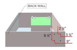
**Note:** It may be easier to drill the 5/16" holes from the back side of the battery box, which means the dump bed will need to be raised.
