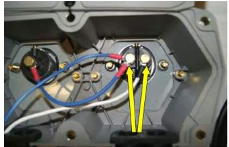
Step 12: Route the 4-gauge 40 ft red and black cables into the dual pole nosebox. Connect the 4-gauge black cable and the Select or Direct ground wire to the negative side of the dual pole receptacle. Connect the
