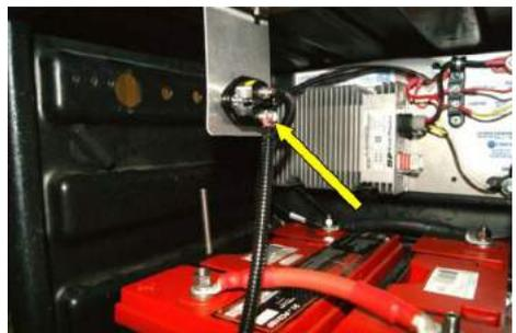
Step 9: Connect the wire marked “30 amp circuit breaker” to the 30 amp resettable circuit breaker and tighten nut. Turn the bracket back to its original position, and re-install the mounting hardware.
