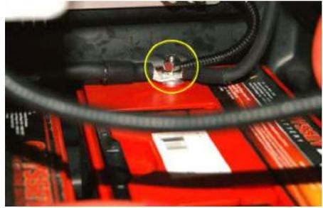
Step 22: Slide the supplied red rubber boot over the 4-gauge red cable and connect this cable to the left side of the 150 amp circuit breaker.
