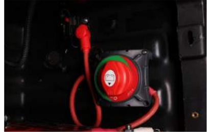
Note: If there is an existing cable from the breaker to the positive post on the battery, remove it, as it is not needed and could hinder proper operation of the system.
