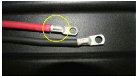
Step 20: Install the red heat shrink to the crimp area of the red cable and the black heat shrink to the crimp area of the black cable. Apply heat to both pieces to seal the connection.
