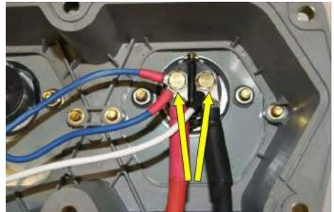
4-gauge red cable and the Select or Direct dual pole positive wires to the positive side of the dual pole receptacle. Tighten bolts, and re-install dual pole nosebox on the trailer.
