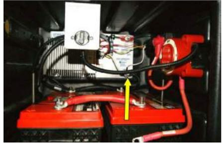
Step 10: Connect the 4-gauge red wire from the 1-2 Switch marked “Liftgate Battery (+)” to the liftgate battery positive post. Install nut and tighten.
