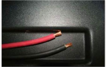
Step 19: Install the 1/4 inch ring terminal on the 4-gauge red cable and the 3/8 inch ring terminal on the black cable. Crimp the connections.
