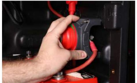
**Step 4:** Push the bolts through the battery box.
