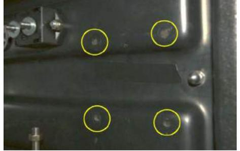
**Note:** If the 1-2 Switch mounting holes do not exist, use the 1-2 Switch as a template to drill these holes.
