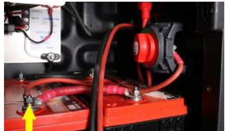
Step 8: Remove two of the 30 amp resettable circuit breaker mounting bolts so that the bracket can be turned to access the back side. Remove the output wire from the 30 amp resettable circuit breaker and discard wire.
