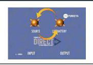
Excessive Voltage Drop - Tractor is running and the voltage is above 13.8 volts. The controller turns on the DC/DC converter and current starts to flow. If the voltage drops below 10.5 volts, the controller will tell the DC/DC converter to turn off. What the operator will see is the Source and Lift Battery go Solid Green, then both LEDs will toggle orange for a few seconds. The cycle then repeats. Note: Low voltage shut off in the first 5 minutes is 9.5 volts.
