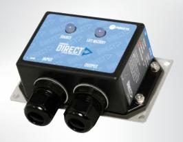
The Direct<sup>™</sup> single-source liftgate charging system boosts voltage through a DC/DC converter to fully charge liftgate batteries faster and overcome voltage drop from the tractor to the liftgate batteries. Draws power from either a stinger cord (dual or single pole) or a 7-Way aux pin.
