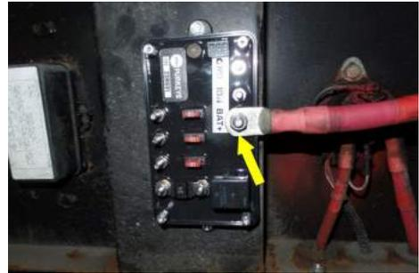
Step 6: Locate vehicle ignition source and run a 14-gauge wire\* from it to the ignition (IGN) stud on the LVD.
