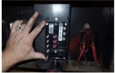
Step 5: Connect the constant power cable to the battery positive (BAT+) post on the LVD.
