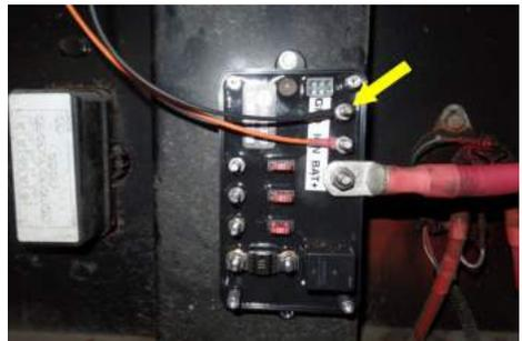
Step 8: Connect an output wire (not included) from the LVD 40 amp main output stud to location where the constant power cable was removed in step 3 (this is typically on a power distribution block).
