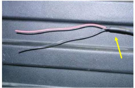
Step 8: Strip 3/8 inch of insulation off both red and black wires.
