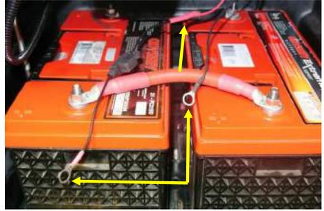
Step 10: Attached the 2 amp fuse holder to liftgate battery positive and the black ground wire to the liftgate battery negative.
