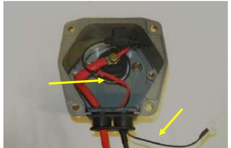
**IMPORTANT:** The chassis ground wire must be attached to a good chassis ground.
