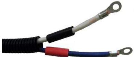
Step 5: Solder then position the heat shrink over the crimps and apply heat to the 2 terminals.
