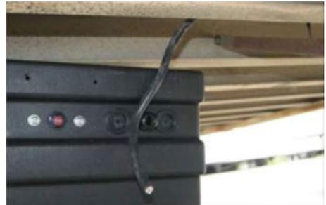
Note: Ensure that the 4-conductor jacketed wire enters the liftgate battery box through a dome nut or rubber grommet to prevent chaffing the wire, which could result in possible electrical short in the system.
