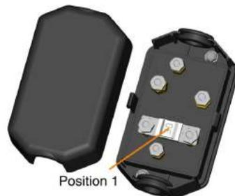
Note: If the 30 amp midi fuse is not positioned correctly, the reefer unit will not function properly as an input source for the Select Liftgate Charging System.
