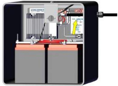
**Note:** If your battery box includes a slide-out tray, include enough slack to allow the tray to fully extend without tugging the wire connections.
