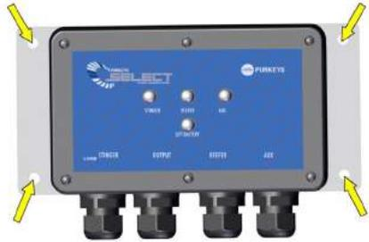
NOTE: Do not block the LED status decal on the side of the Select when mounting the Select Controller.
