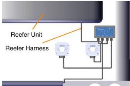
Note: Place the cable clamps along the reefer harness every 6 inches to ensure proper support for the cable. Avoid sharp edges and possible chaffing points.
