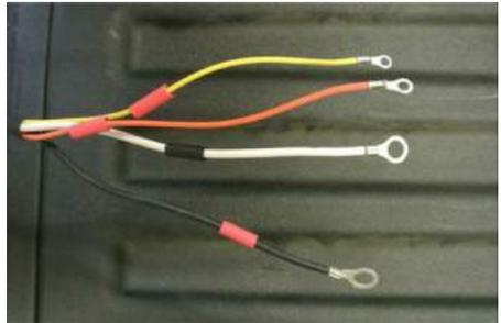
Step 11: Position the heat shrink over the crimps and apply heat to the 4 terminals.
