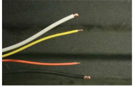
Step 9: Slide the supplied red inch heat shrink over the orange, yellow, and black wires. Slide the supplied black inch heat shrink over the white wire.
