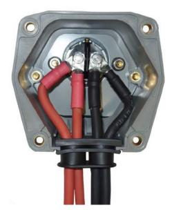
Step 6: Attach the positive charge cable to the positive side of the dual pole receptacle. Attach the negative charge cable to the negative side of the dual pole receptacle.
