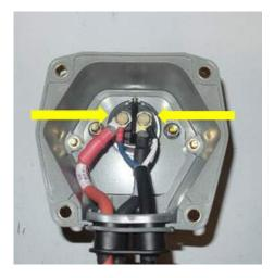
Step 6: Route the red charge cable and black cable on the front of the trailer and under the header plate using the access points and pathways provided by the trailer manufacturer. Securely attach cabling with the holddowns and fasteners provided.
