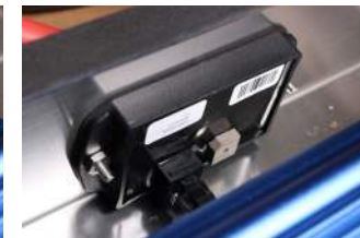
800-220 TAPS Controller LVD Set to 11.9 V
