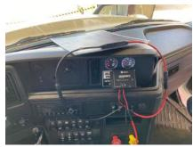
Step 3: Connect the power plug adapter included in the kit to the Solar Dash controller.
