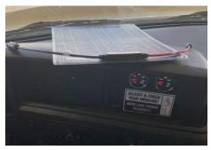
Step 2: Plug the 20-watt solar panel into the solar controller via the MC4 connectors. Connectors can only be plugged in one way.
