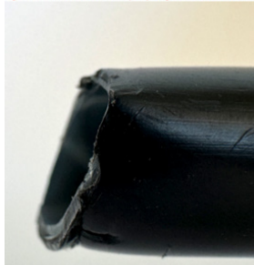
Nylon brake hose cut improperly with side cutters
