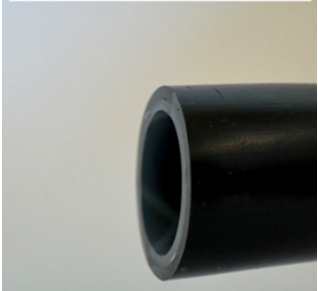
Nylon brake hose properly cut with sharp blade
